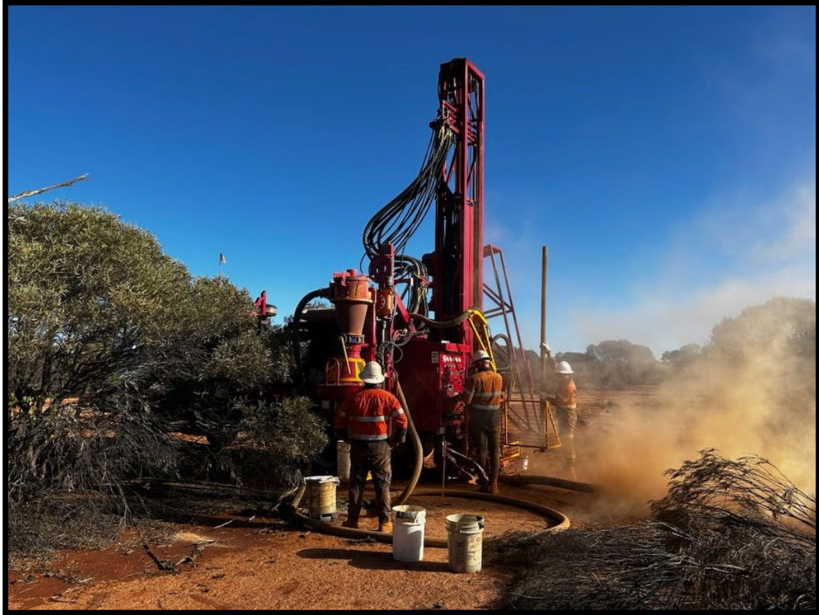
Figure 3: Fenceline aircore drilling in progress at Revere
