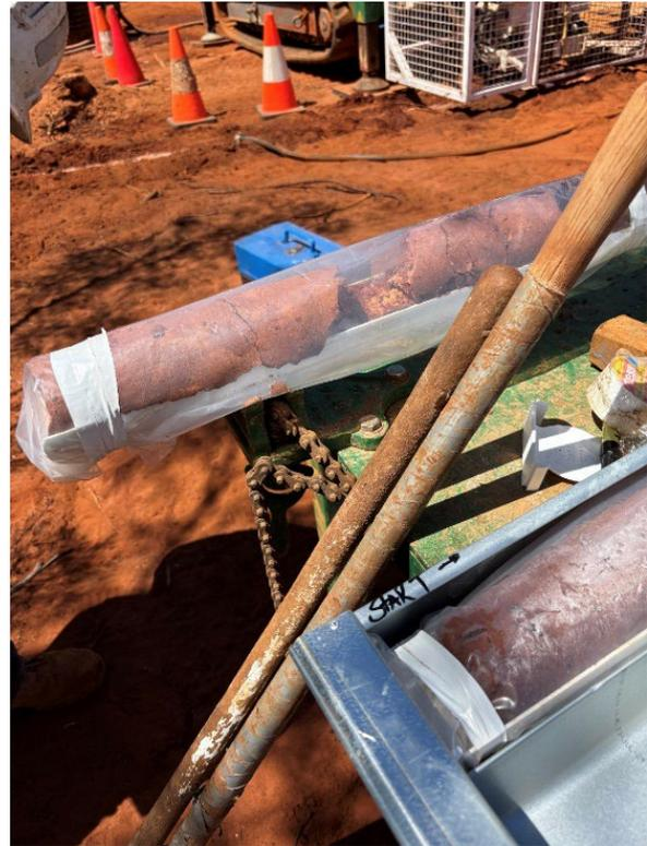
Figure 7: Diamond core drilling is underway at Goongarrie Hub, with the core wrapped in plastic to preserve density/moisture for measurement. An example of a Magnesium Neutraliser is shown, but assay results are not yet available, so no comment can be made on acid neutralisation or nickel-cobalt grade.
