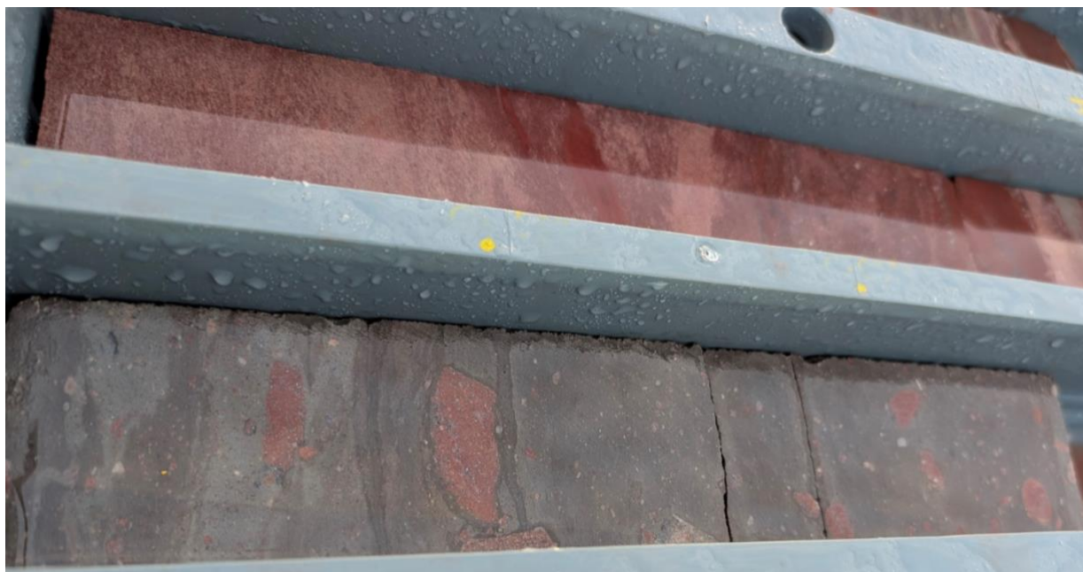
Figure 1 Reducing black mud supported conglomerate in drillhole DD25EB0038, moderately mineralised with disseminated chalcocite.
