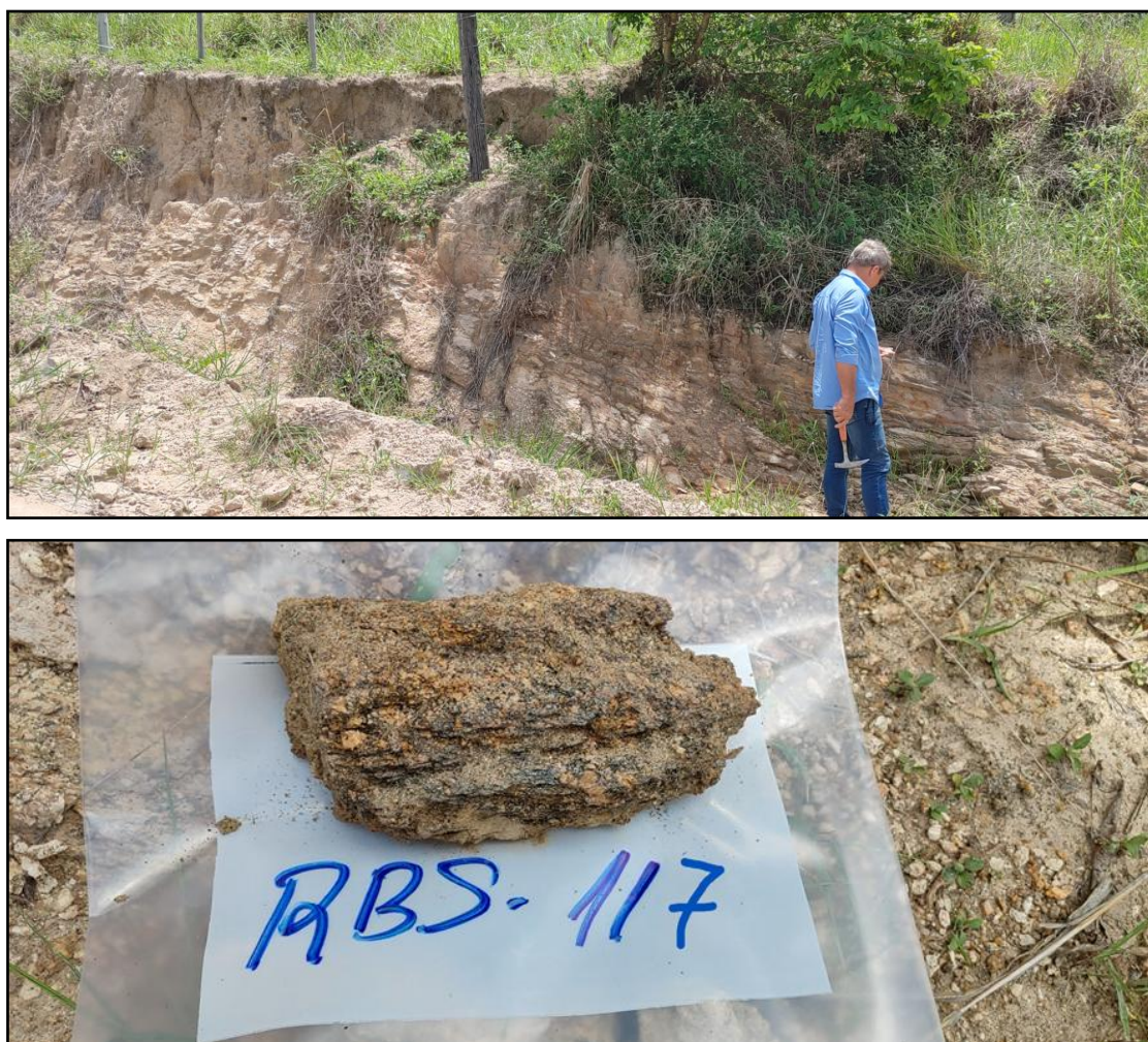
Figure 2. Sample RBS-117 collected from an exposed weathering profile with 25,817ppm TREO (25% MREO), 9.3%TiO 2 and 8,619ppm ZrO 2 .
