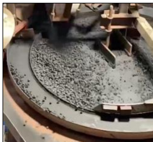
Picture 1. Green Ball manufacture in pelletising disc
