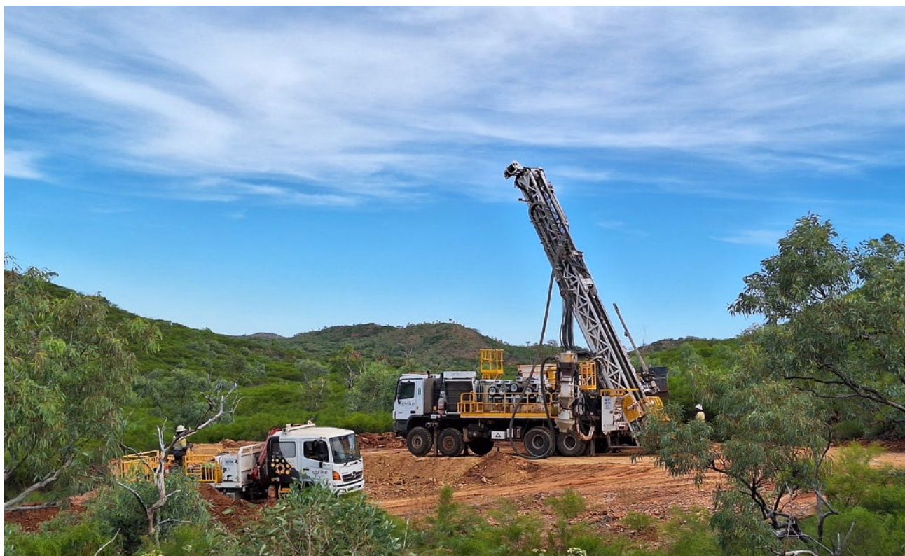
Figure 1. Reverse Circulation drilling rig operating at Mount Mascotte
