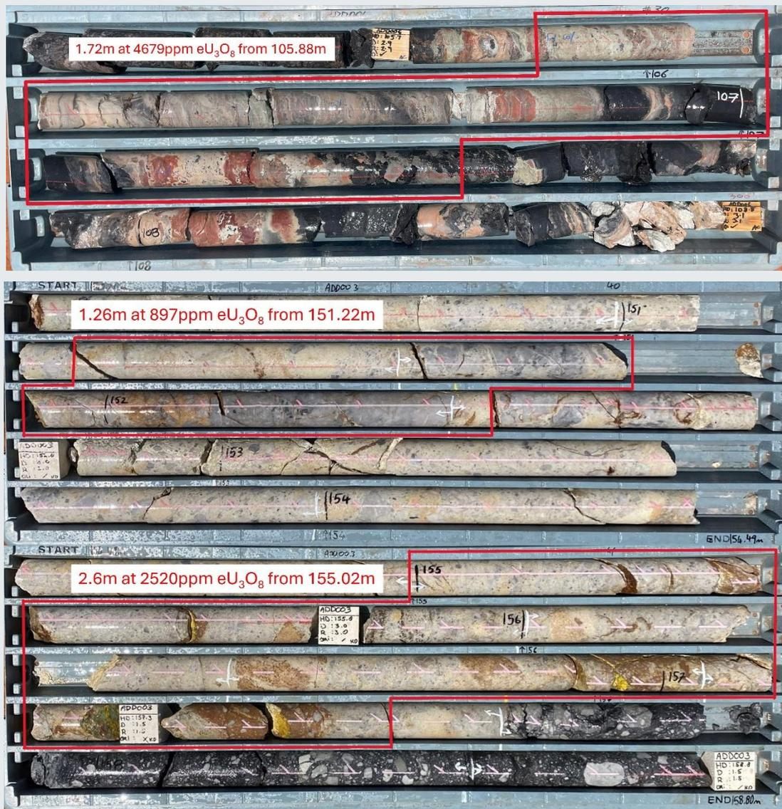
Figure 8: Top image – Drill core photo highlighting the high-grade uranium mineralisation in talus unit in diamond drill hole ADD006.<sup>2</sup>
