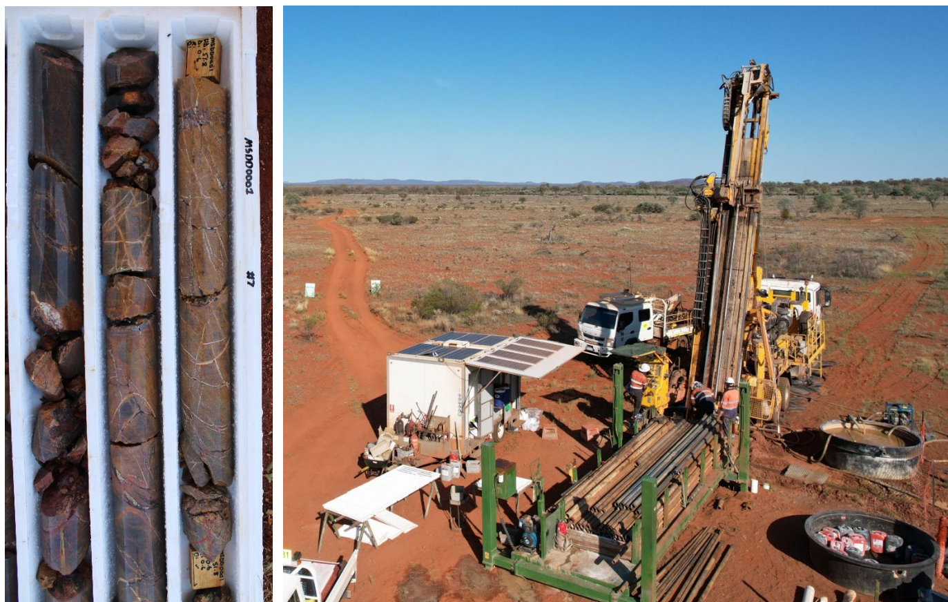
Figure 6. Hydrothermal veining and likely REE mineralisation from diamond hole MSDD0001, Duchess REE Prospect, Mount Squires Project, October 2024.
