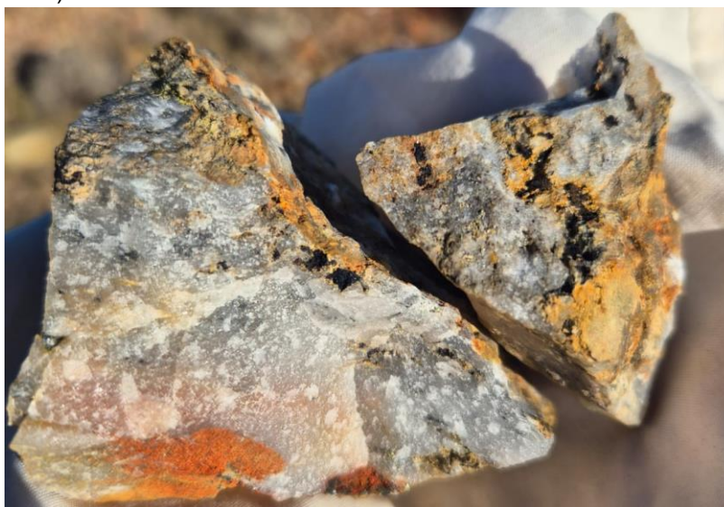
Figure 5: Photograph of sample LY04 of quartz veins with gossanous disseminated sulphide that assays 114.4 g/t Au, 45.8 g/t Ag, 0.33% Cu, 0.25% Pb and 0.53% Zn.
