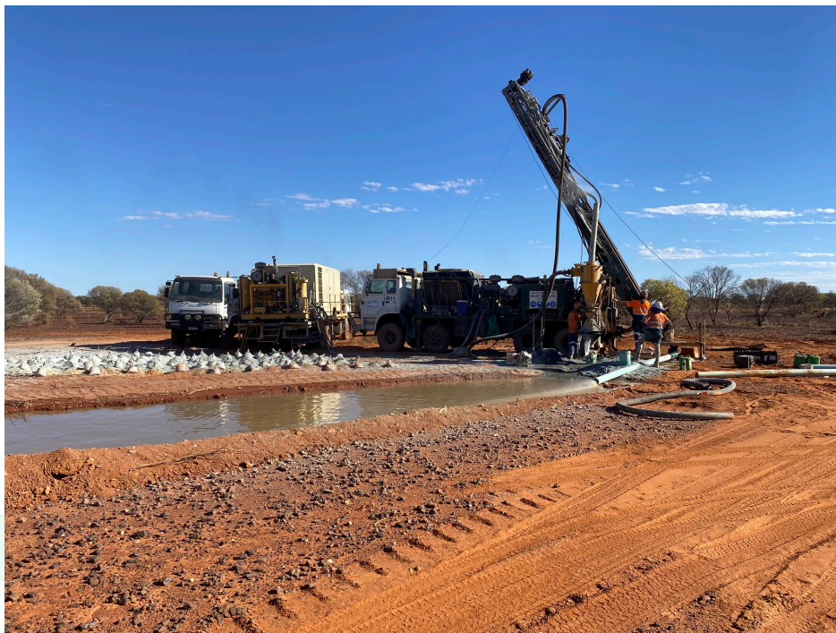
Figure 1: NDRC Pty Ltd reverse circulation drilling rig in action at Byro South
