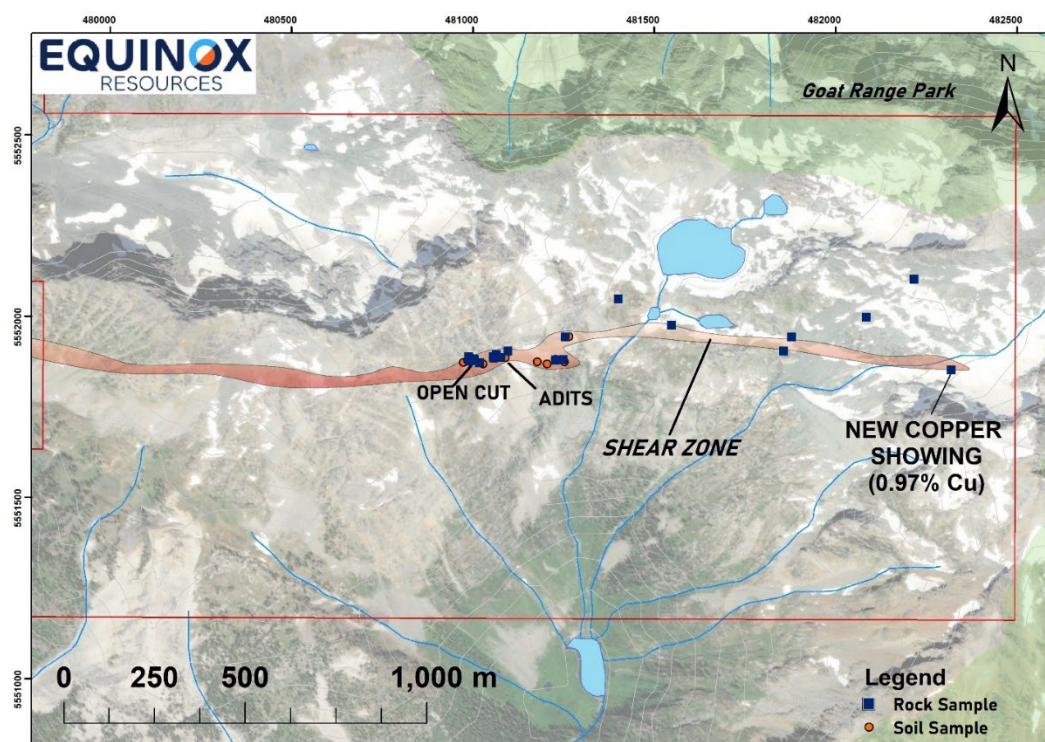
Figure 7: Geological map of the Alturas Antimony Project showing the 1.5-kilometre-long stibnite-bearing shear zone, location of historical open cuts, underground adits, and newly identified copper mineralisation (0.97% Cu).
