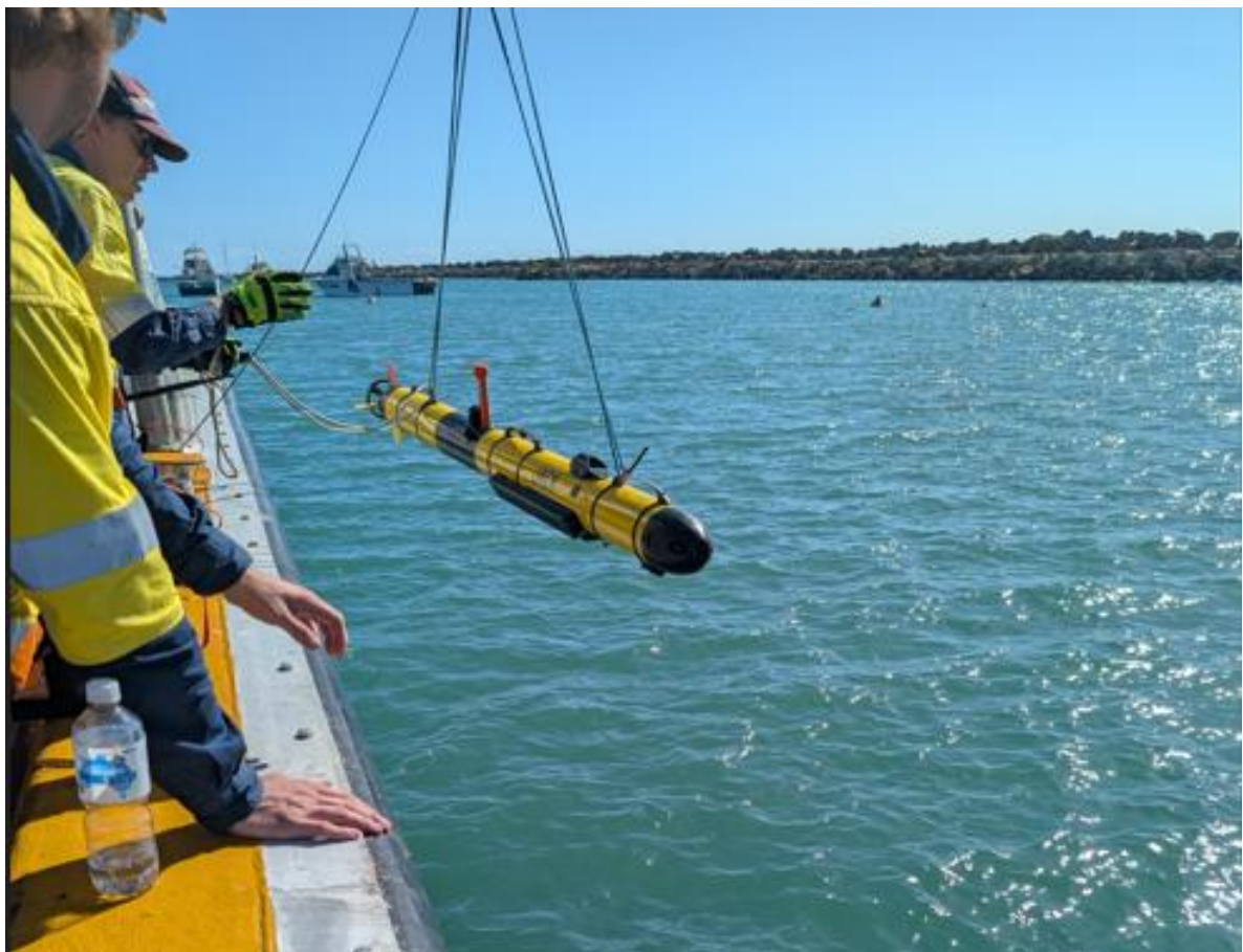
AUV being deployed from operation vessel
