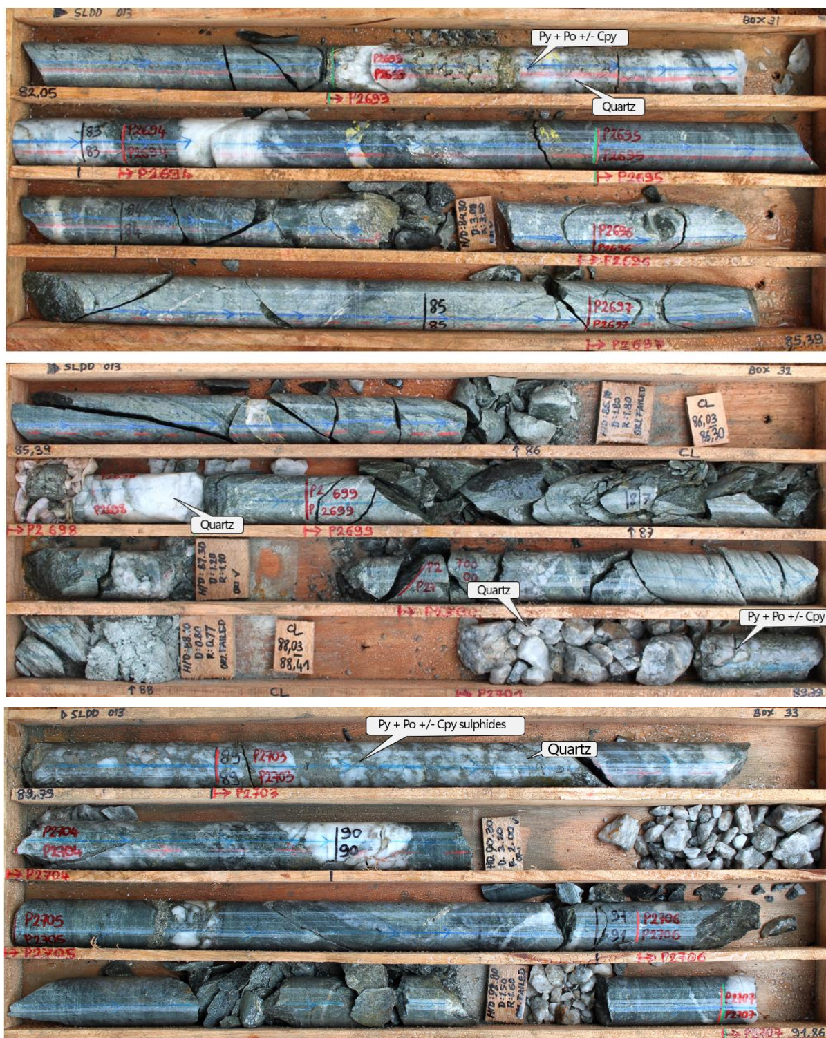
Figure 8: Veining and sulphides in hole SLDD013 showing quartz veining (~32%) associated with pyrite (Py - 1 to 25%), pyrrhotite (Po - trace to 10%) and chalcopyrite (Cpy - trace to 3%) seen from 82.3 to 92.5m (refer Table 2).
