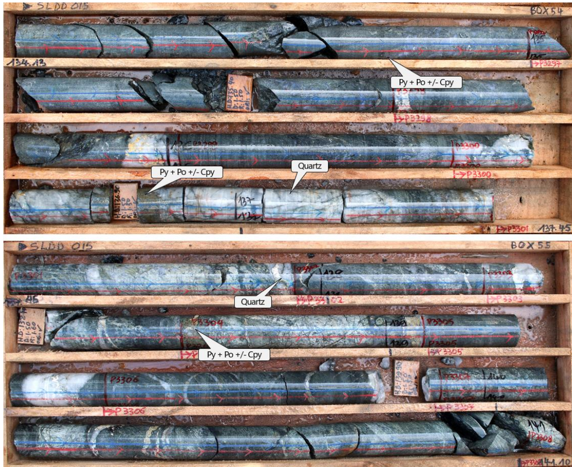
Figure 9: Veining and sulphides in hole SLDD015 showing quartz veining (~30%) associated with pyrite (Py - 1 to 10%), pyrrhotite (Po - trace to 3%) and chalcopyrite (Cpy - trace to 1%) seen from 135.6m to 141.4m (refer Table 2).
