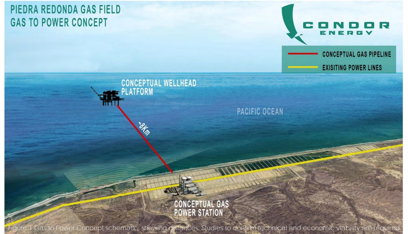
Figure 1 Gas to Power Concept schematic, showing distances. Studies to confirm technical and economic viability are required.
