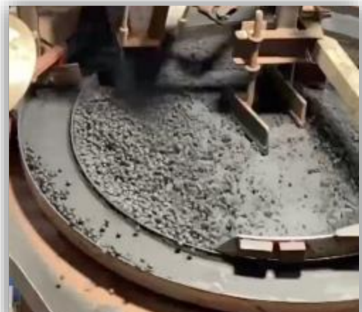
Picture 1. Green Ball manufacture in pelletising disc
