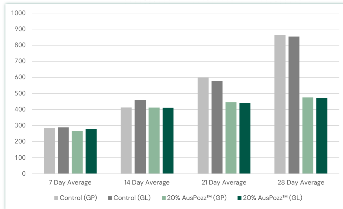
40MPa Shrinkage (Microstrains)
