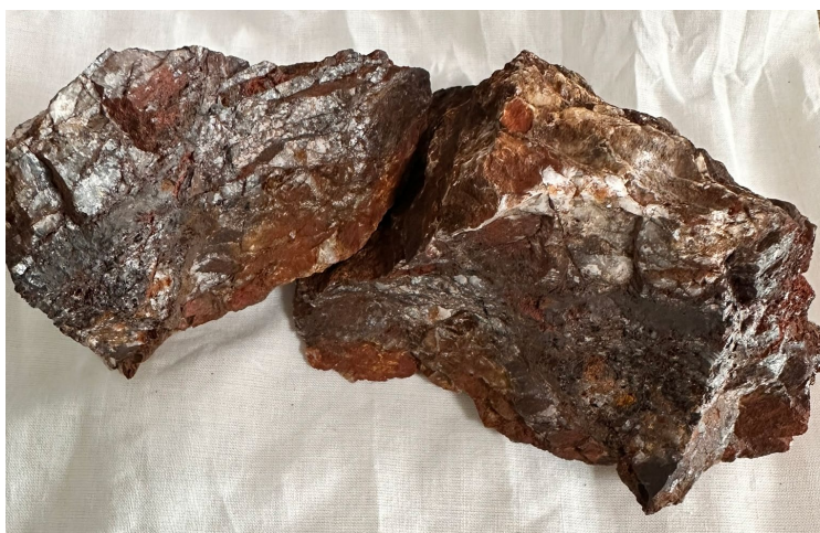
Figure 1: Gossanous quartz vein (MP25_006) which assayed 10.15g/t Au.
