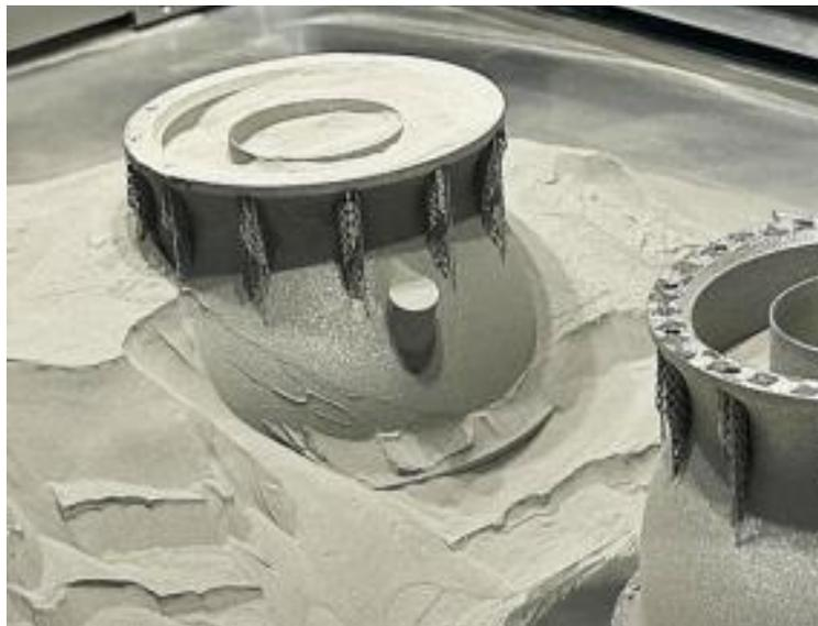
*Printed Engine Parts in the Printing Chamber*
