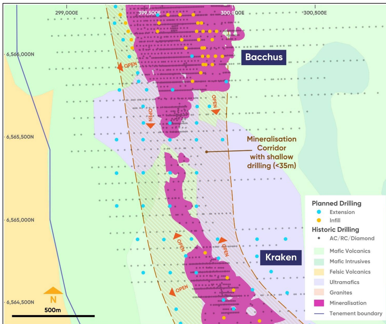
Figure 4 - Bacchus–Kraken trend with modelled mineralisation (plan projection) and proposed drill collars
