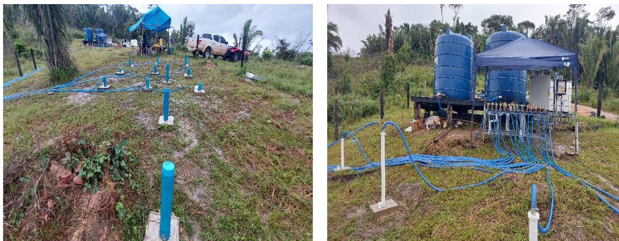
Figure 1. view of the water storage and magnesium sulphate storage tanks piped to injection holes designed and drilled to optimise and test solution permeability.
