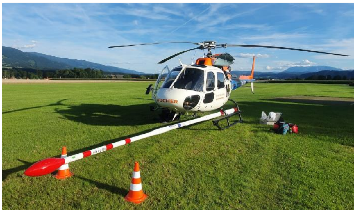
Figure 2: Nose boom magnetic and radiometric configuration on helicopter.
