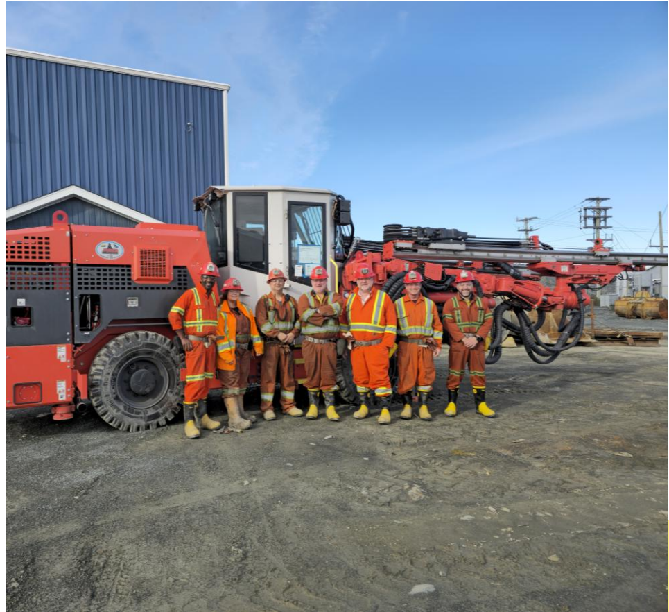
Twin boom jumbo at the Ming Mine
