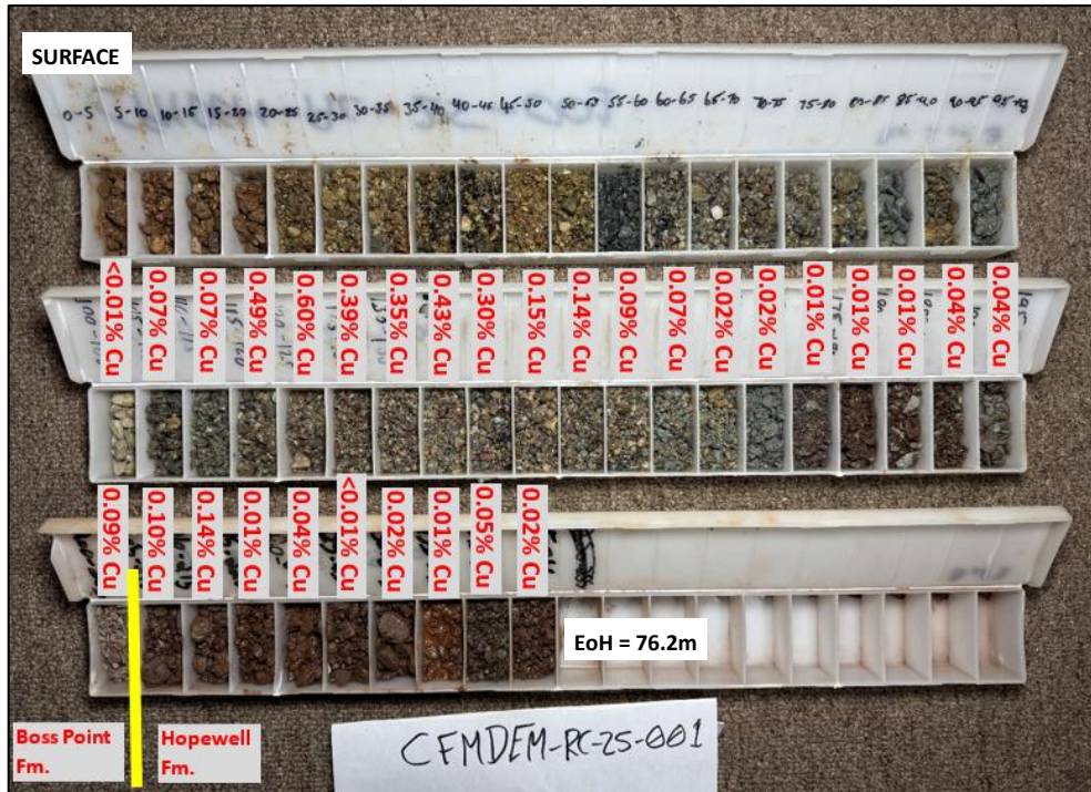
Figure 2. RC chip trays from CFMDEM-RC-25-001 annotated with assay results.
