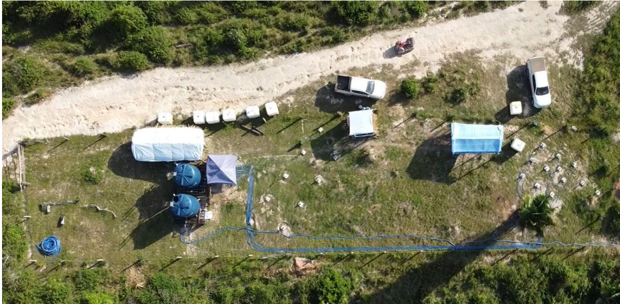
Figure 2. aerial view of the ISR setup, injection and extraction holes and associated infrastructure.
