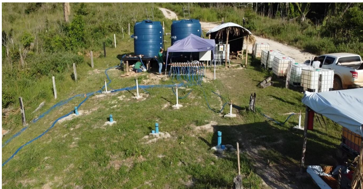
Figure 1. view of the water storage tanks piped to injection holes designed and drilled to optimise and test solution permeability.
