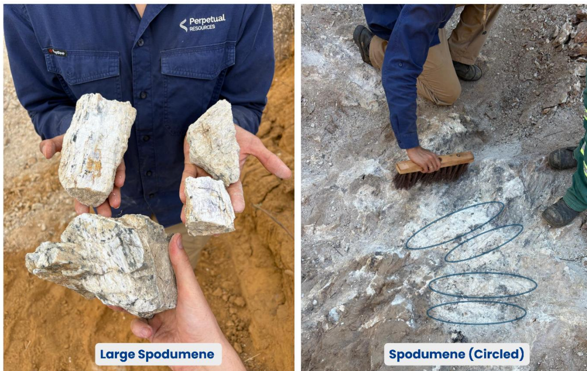
Figure 2: Spodumene encountered during pre-drill access road preparations at Igrejinha.
