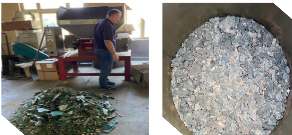
Figure 2: Photo of (L) original E-Waste PCB waste & (R) metal rich char (E-Waste with plastics removed by separate process)
