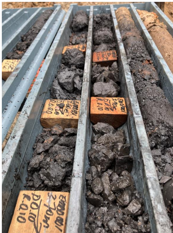
Figure 1: LEFT: EMDD001 core from 1.35 to 3.7m (Tray 1) RIGHT: Exploration Manager Steve Warriner at trench EMT01 Both the core and the trench contained 95% manganese oxides and 5% silicious manganese oxides
