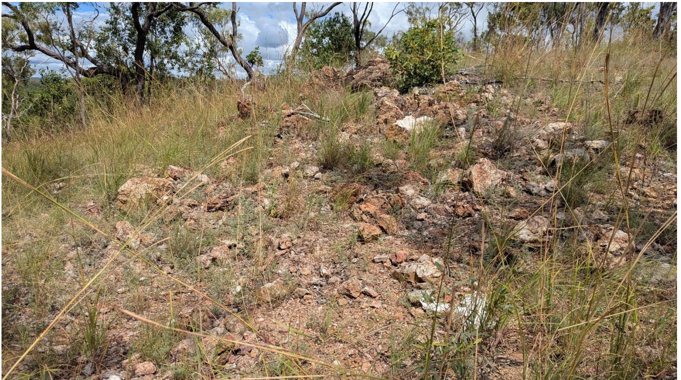
Figure 2. Outcropping quartz stockwork at a previously unsampled site south of the historic Bouncer Prospect workings. Rock chip sample IRX00011 returned an assay of 1.95 g/t Au, confirming gold mineralisation in this newly identified area.
