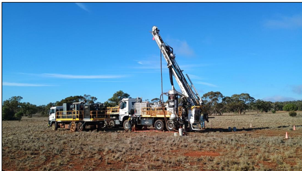
Figure 2: RC drill rig collaring on the first hole of the new program.
