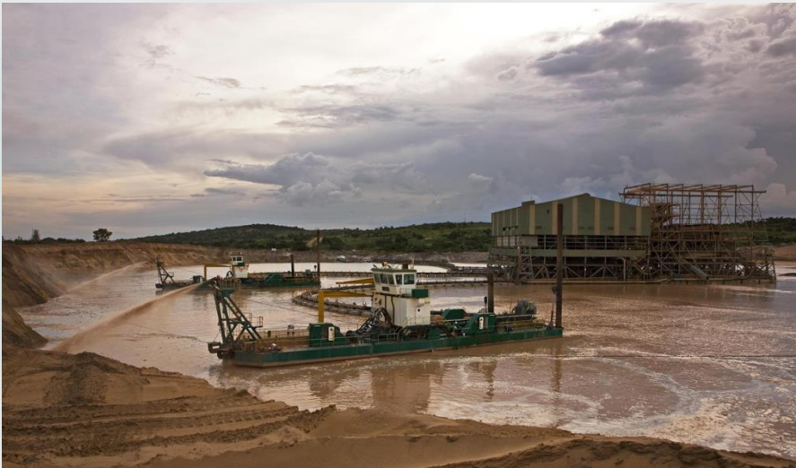
Above: Example of two mineral dredges and floating wet concentrator
