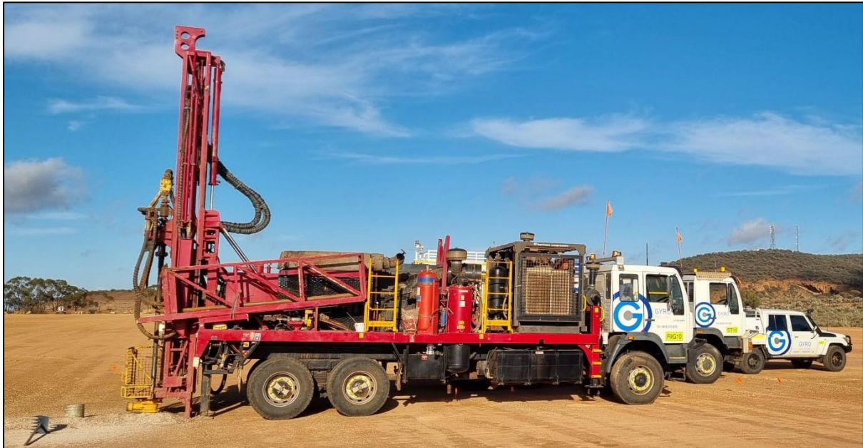
Figure 1. Aircore drill rig for the Beatty Park Sth drill program.
