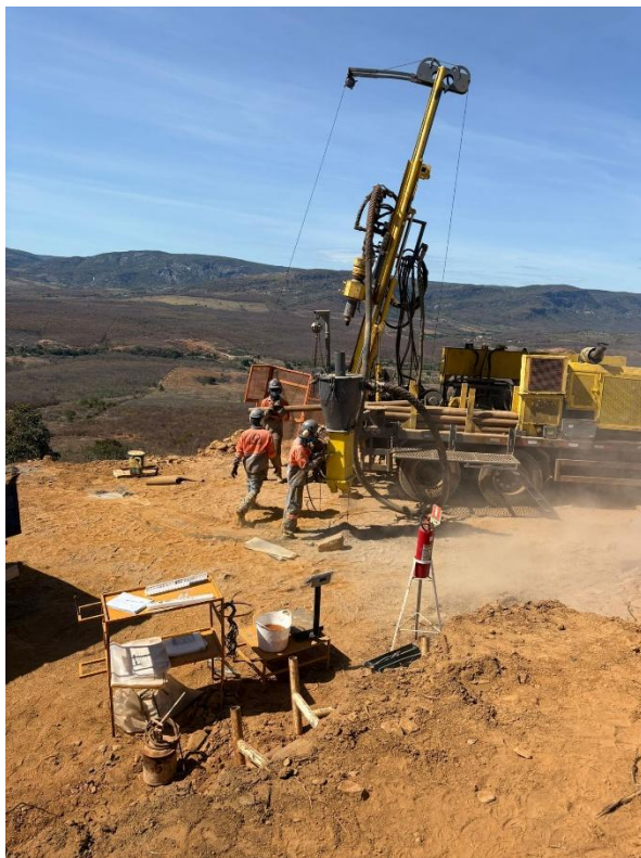
Figure 1: Image showing Reverse Circulation (RC) drilling underway at "Target 1" at the Igrejinha Lithium Project.
