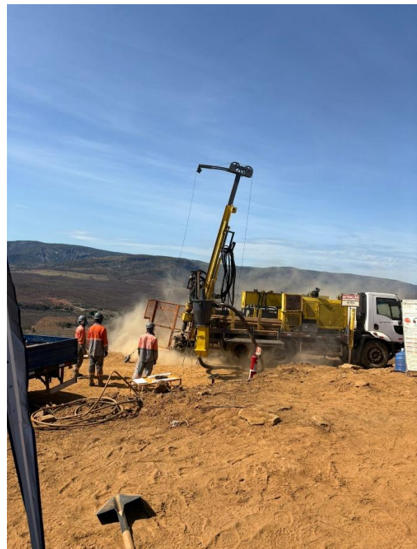
Figure 1: Image showing Reverse Circulation (RC) drilling underway at "Target 1" at the Igrejinha Lithium Project.
