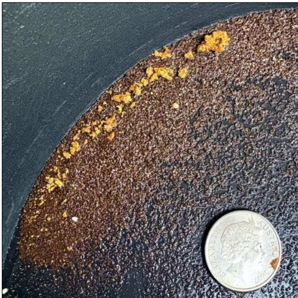
Figure 1 - Gold recovered from panning the bulk 1m sample for the interval 37-38m in drill hole INRC25073, which reported 1m at 356g/t gold. Coin for scale is approximately 20mm in diameter. For drillhole information refer to Table 1.
