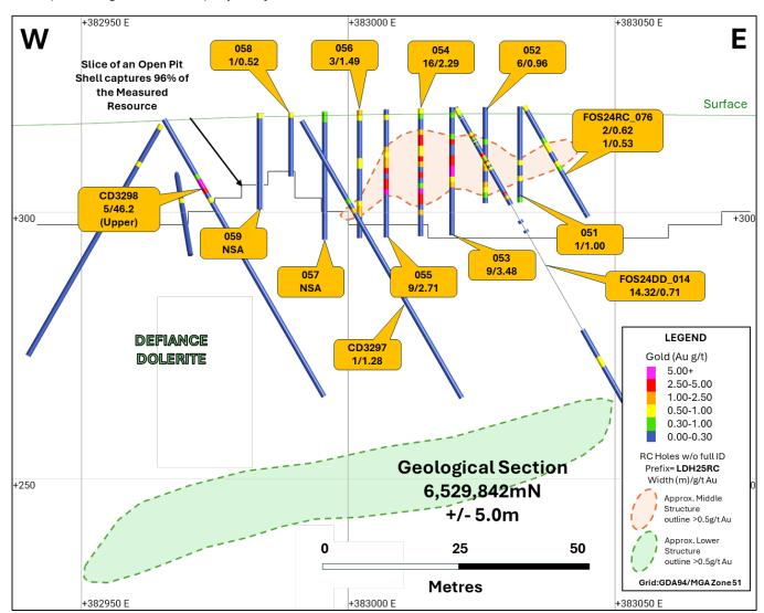
Figure 5: Geological cross section 6,529,842mN - Middle Structure - showing a slice through a potential open pit shell.
