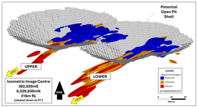
**Figure 8**: Isometric view, looking down and toward the NNE, of the Lady Herial gold deposit illustrating the Upper, Lower and Middle Structures coloured by Mineral Resource classification categories.
