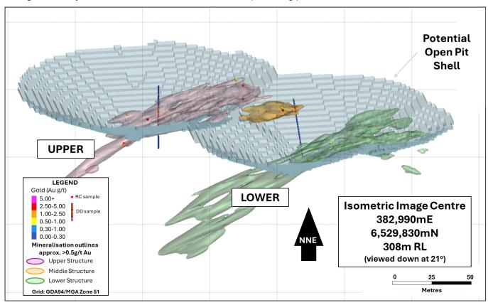
**Figure 10**: Isometric view of the Lady Herial system showing location of RC (spheres) and DD (traces) drill holes from which metallurgical samples were sourced relative to the depth profile of the deposit.
