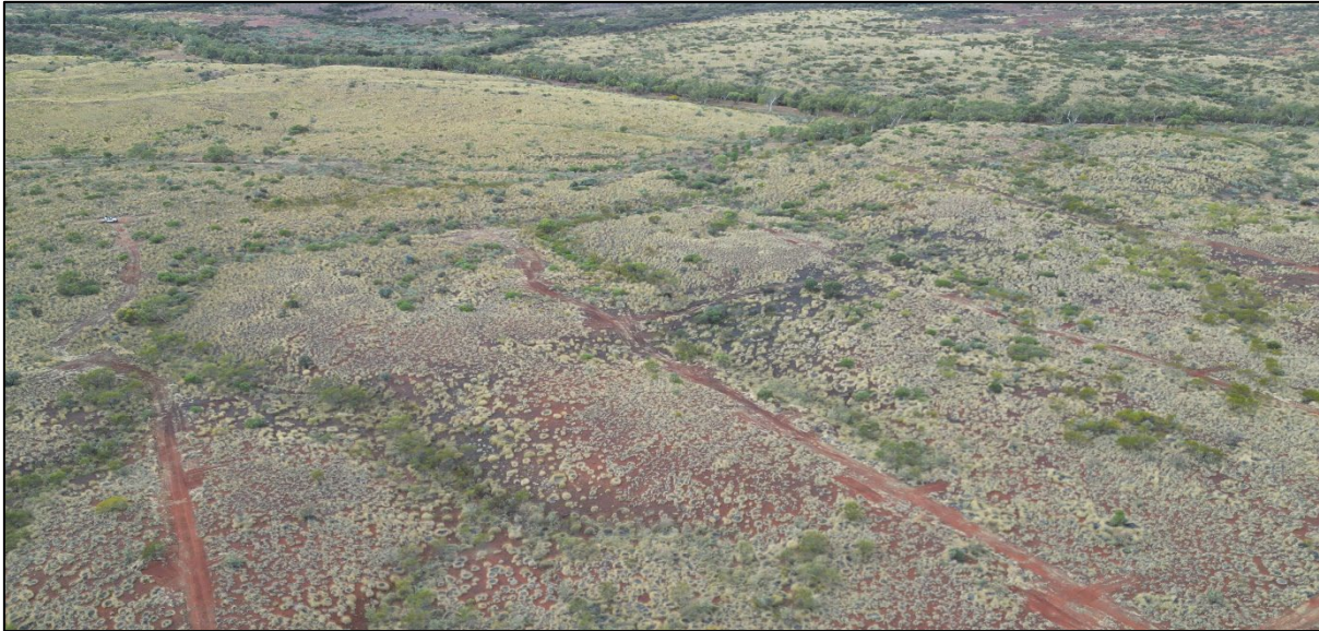
Figure 3. Drone image looking to the southeast highlighting the east dipping manganese horizon to be tested as part of this phase 2 RC drill program.
