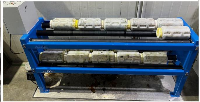
IBRT is used to simulate the leaching mechanism inherent in heap leaching and is the precursor to column leach testwork for additional heap leach parameter establishment. Each bottle is agitated (turned on rollers) for five minutes every hour, such that diffusion is the dominant mechanism for lixiviant transfer into the crushed ore. This is the same mechanism that dominates in heap leaching.
