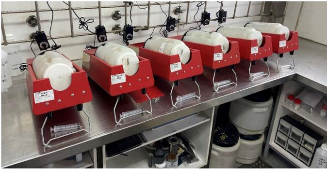
**Figure 3: Dubbo Project Phase B – intermittent bottle roll leach tests**
