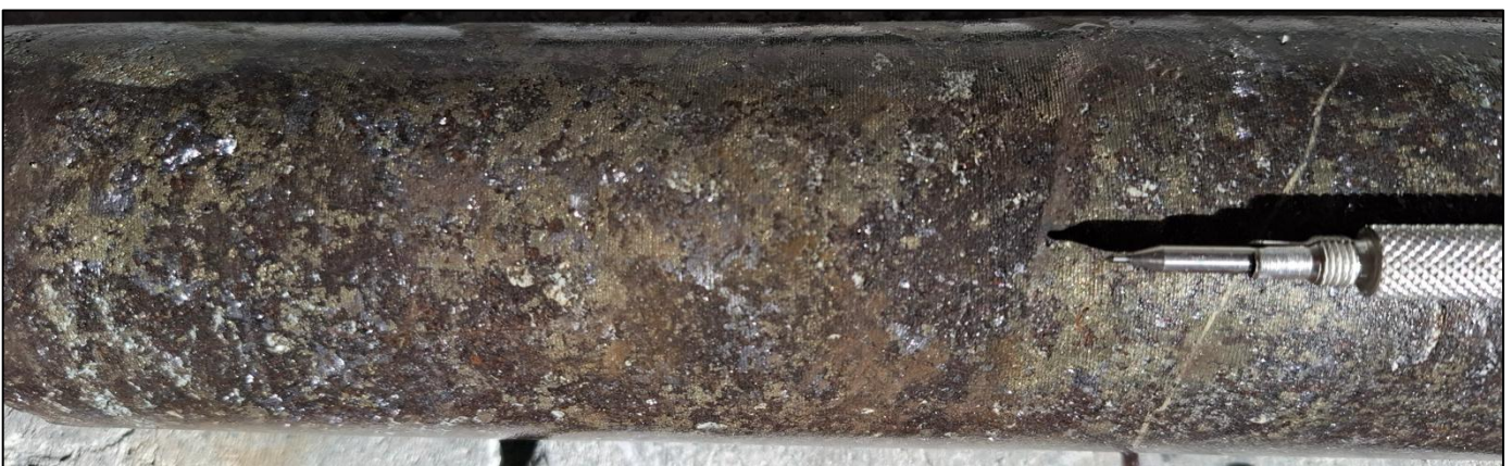
Figure 5: Core photo of skarn-hosted mineralisation with massive sphalerite and galena from 515.6m in ZRSD25179A – 0.4g/t Au, 0.2% Cu, 12.4% Pb, 13.9% Zn and 90.7g/t Ag (11.1g/t AuEq 2 ).
