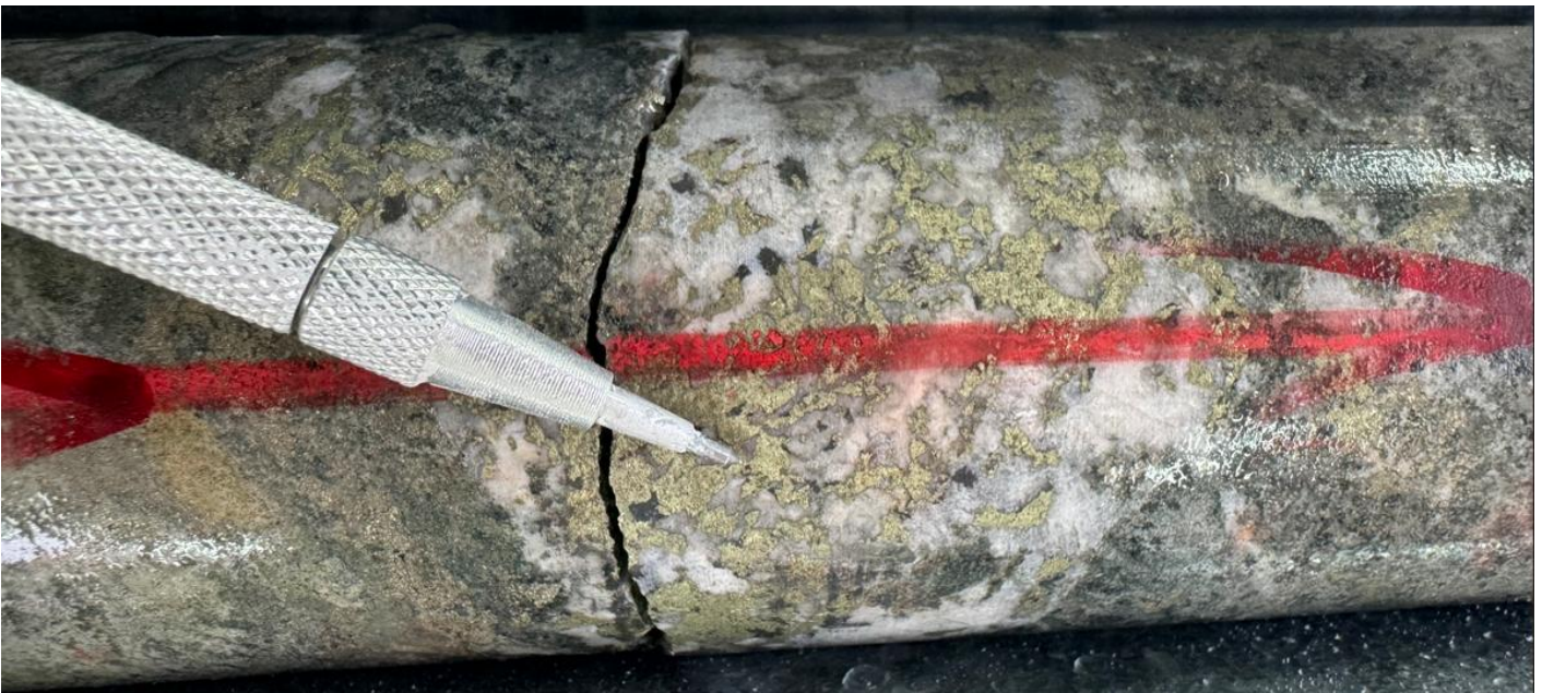
Figure 7: Core photo of skarn-hosted mineralisation with chalcopyrite and pyrite from 456.5m in ZRSD25180 – 3.5g/t Au, 0.5% Cu and 3.3g/t Ag (4.2g/t AuEq 2 ).
