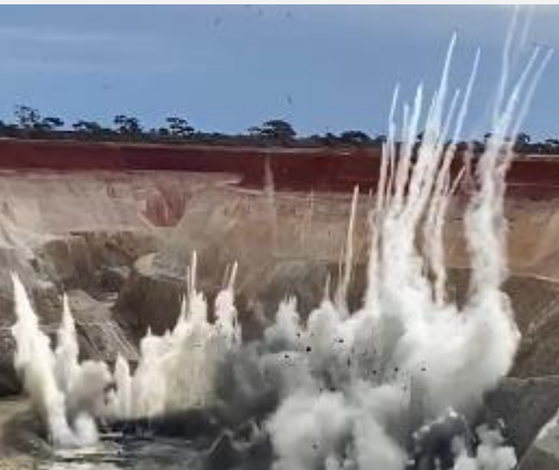
TRADITIONAL PIPING PROCESS WITH POOR BLAST AND OPERATIONAL OUTCOMES
