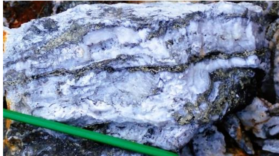
120 Vein (Singha Creek); colloform banded white quartz and sulphides
