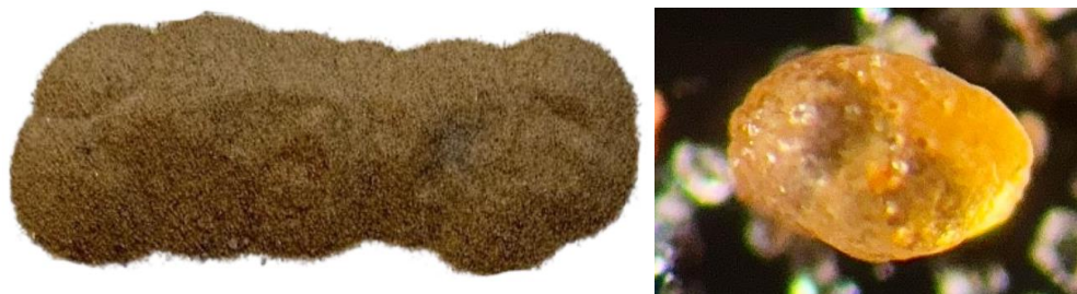
Figure 1: Separated monazite from RE1028 alluvial sample at Minta Est (Refer Appendix 3 for further information).
