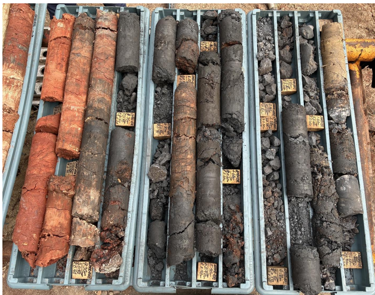
Figure 2: Tray 1 (right) to tray 3 (left) of EMDD002 showing the full intersection of PQ core with visual estimates presented in Table 1
