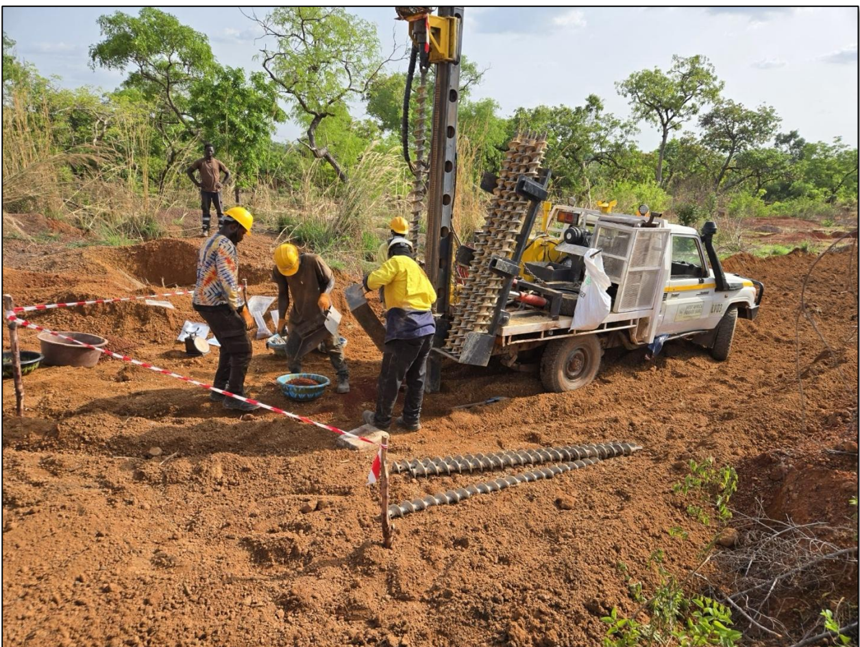
Fig. 2 – Power auger drilling being completed at the Dadjan Gold Project, located in the Siguiri Basin, Guinea.
