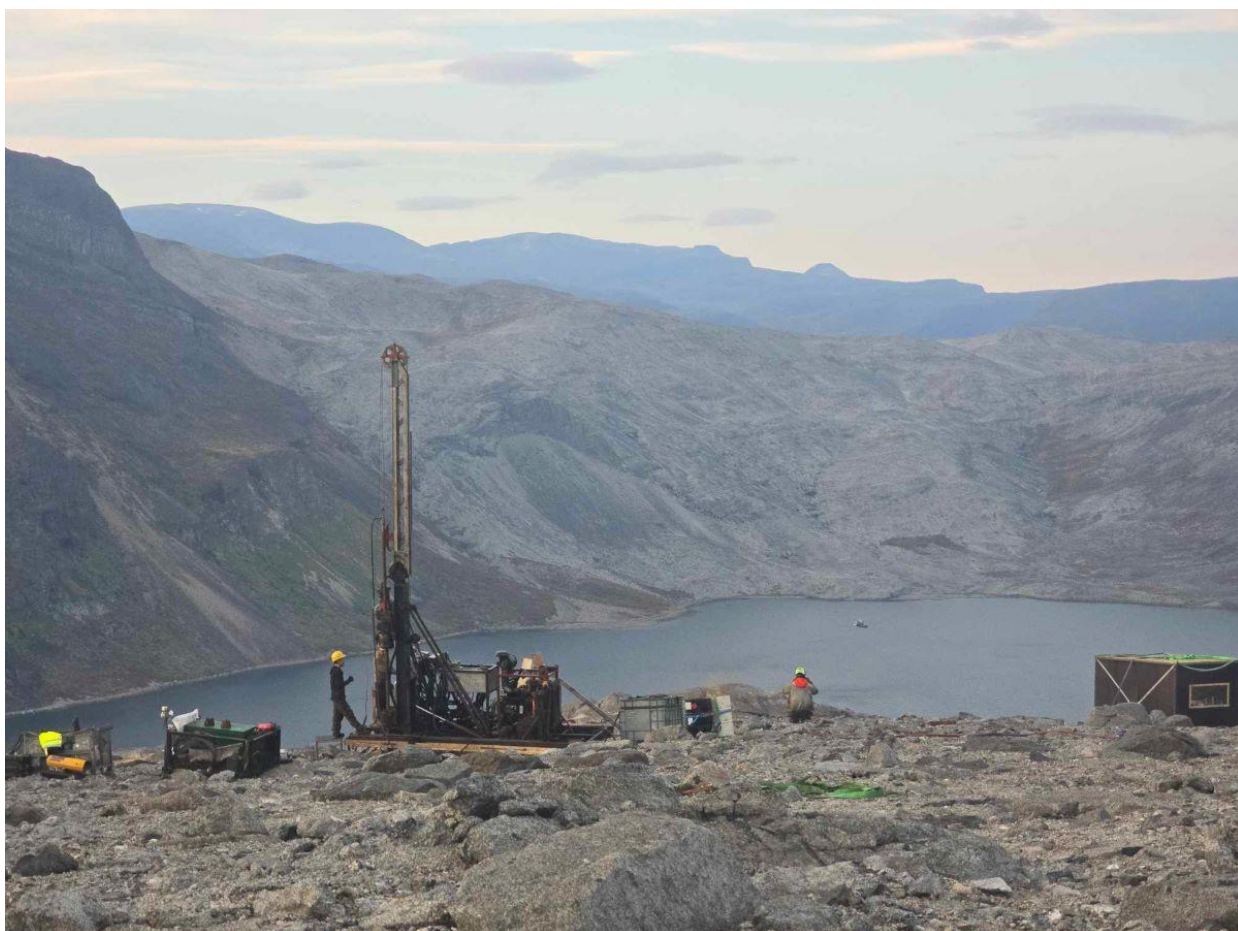
Figure 2 Diamond drilling November 2024 drill collar K-24 within 200m of proposed 2025 program to North-East of and above the Fjord Deposit
