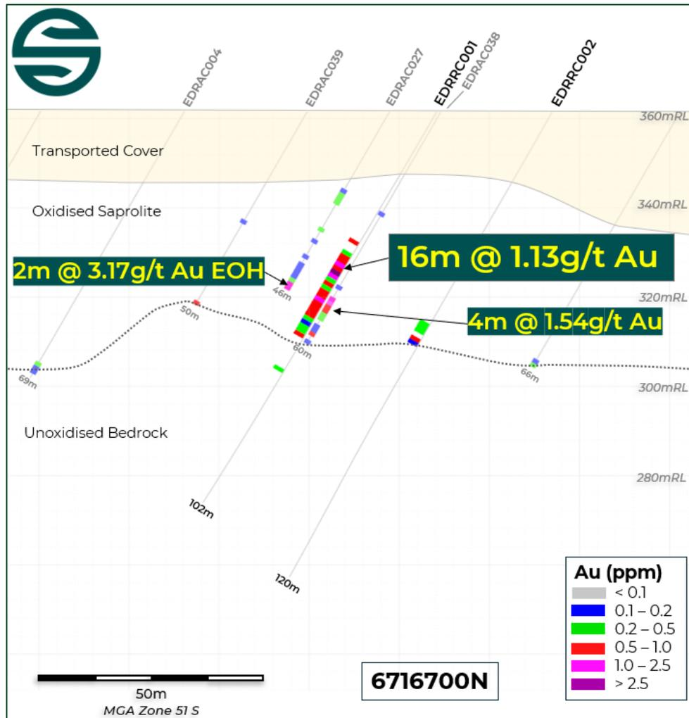
**Figure 2: Edjudina Range cross section 6716700N, showing completed RC drillholes EDRRC001 & EDRRC002 and gold results in composite sampling, aircore drill traces and key downhole gold results also shown.**
