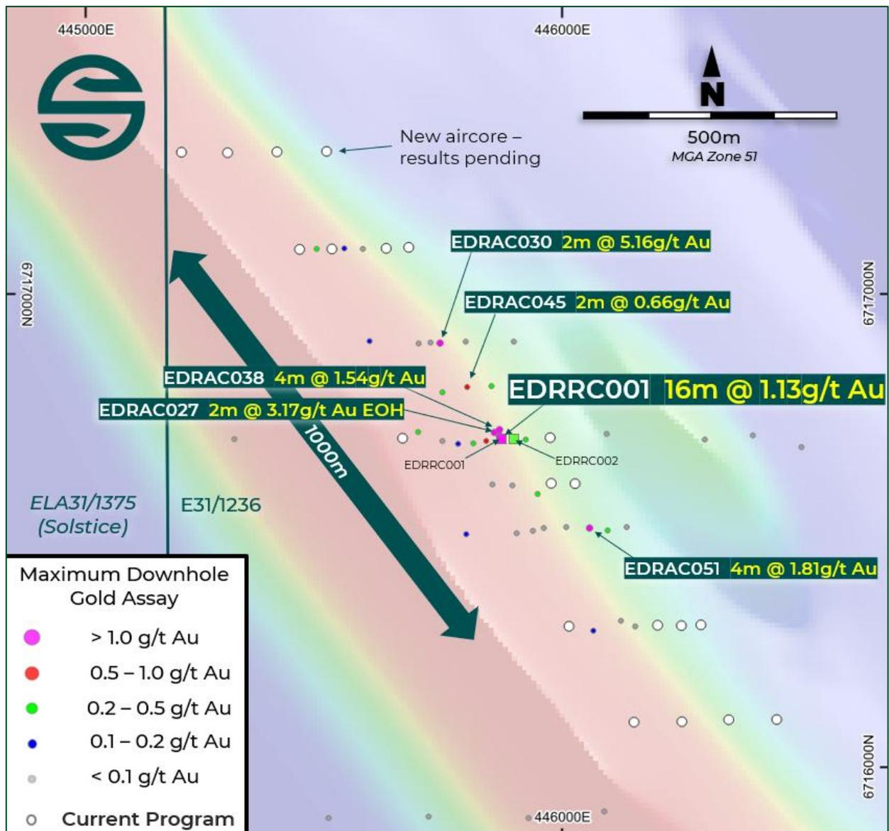
**Figure 1: Edjudina Range Gold Prospect showing aircore drillholes completed in the current program (white circles) on aeromagnetic image, and all previous drillholes coloured for peak down-hole gold values. Significant gold intercepts are labelled.**
