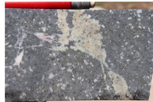
Photo 18 ragged juvenile intrusion clast in magmatic hydrothermal breccia, STDD001, 331.4m.
