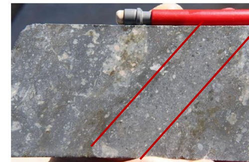
Photo 15 Milled matrix breccia with milled clasts in an illite-pyrite altered rock flour matrix and cross-cutting dyke-like finer grained phase on the right DDH STDD001, 336.6m.
