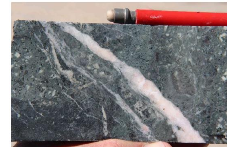
Photo 25 Shear-hosted rhodochrosite vein cuts magmatic hydrothermal breccia, DDH SMTDD001, 386.1m.
