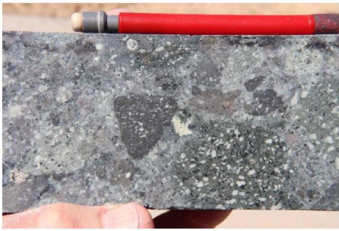
Photo 20 Coarse grained crowded magmatic hydrothermal breccia characterised by milled mixed porphyry clasts. STDD001, 395.8m.
