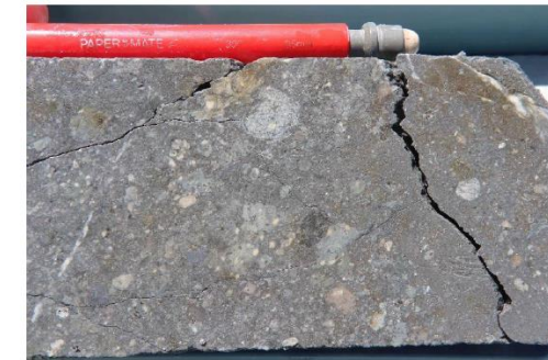
Photo 14 Milled matrix breccia with milled clasts in an illite-pyrite altered rock flour matrix and cross-cutting finer grained phase on the right DDH STDD001, 342.7m.
