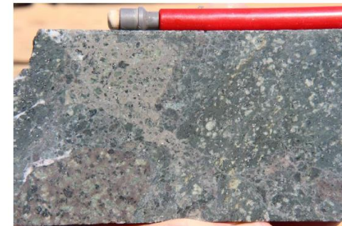
Photo 17 Ragged juvenile intrusion clast within a magmatic hydrothermal breccia, DDH STDD001, 336.8m.
