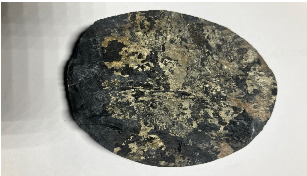
Figure 5. MTCD001 @ 84m. Sulphide-bearing black shale hosting pyrite and pyrrhotite.
