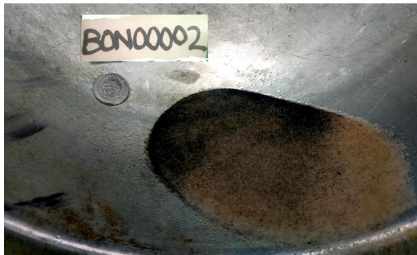
Figure 8: Fine grained HM within a quartz matrix from panned concentrate of a 1m auger interval sampled at GRMAU0007. Cautionary Statement: The visual representation of heavy mineral (HM) and rutile mineralisation shown in this release is based on preliminary visual reconnaissance with no sampling results. Assay results are pending and have not yet been verified through laboratory analysis and expected in August 2025. Investors are cautioned that the information is indicative only and should not be relied upon as a definitive measure of mineralisation or economic potential. Further exploration and analytical testing are required to confirm the extent, grade, and economic viability of the mineralisation.
