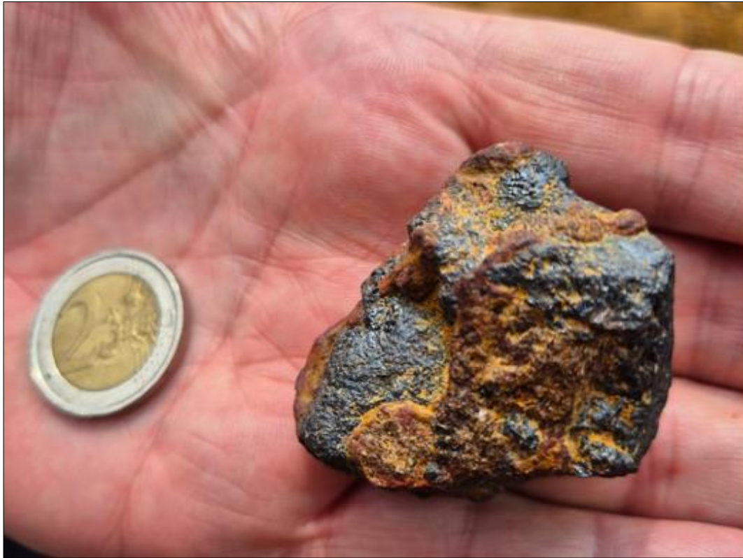
Figure 9: A coarse rutile nugget (~4cm) with partial thin secondary ferricrete coating was recovered from residual regolith comprising mainly fine-grained, iron-rich soil and clay near a road cutting at sample site GRMAU0012. Cautionary Statement: The visual representation of heavy mineral (HM) and rutile mineralisation shown in this release is based on preliminary visual reconnaissance with no sampling results. Assay results are pending and have not yet been verified through laboratory analysis and expected in August 2025. Investors are cautioned that the information is indicative only and should not be relied upon as a definitive measure of mineralisation or economic potential. Further exploration and analytical testing are required to confirm the extent, grade, and economic viability of the mineralisation.
