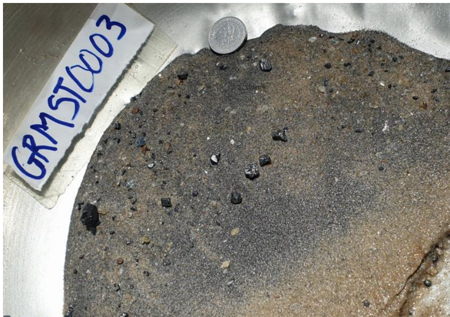
Figure 6: Fine grained HM and rutile grains and nuggets (~1-5mm) with accessory garnets, quartz and kyanite from panned concentrate of a stream sediment sample collected from GRMST0003. Cautionary Statement: The visual representation of heavy mineral (HM) and rutile mineralisation shown in this release is based on preliminary visual reconnaissance with no sampling results. Assay results are pending and have not yet been verified through laboratory analysis and expected in August 2025. Investors are cautioned that the information is indicative only and should not be relied upon as a definitive measure of mineralisation or economic potential. Further exploration and analytical testing are required to confirm the extent, grade, and economic viability of the mineralisation.
