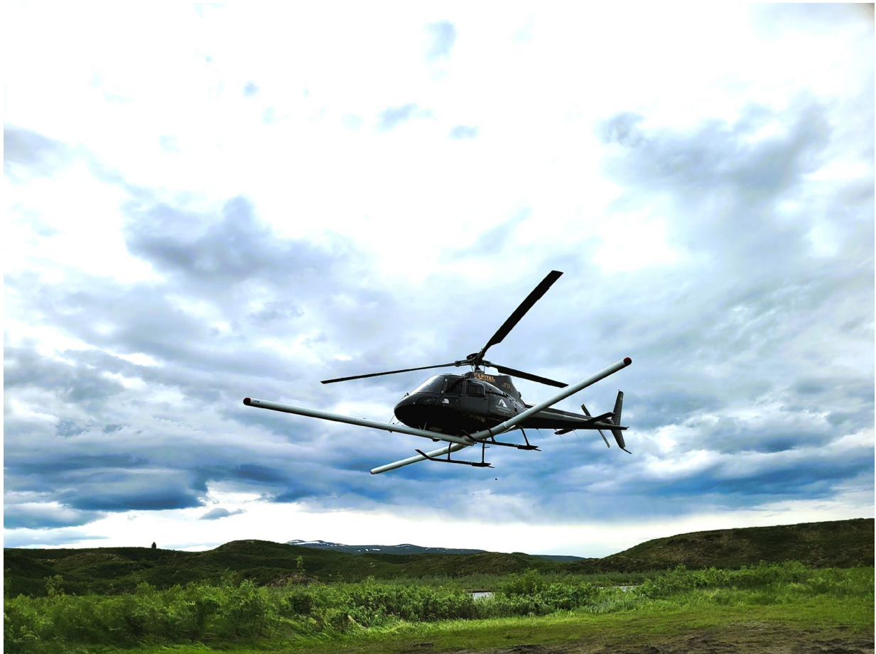
Figure 1. Airborne Geophysics surveying at 50 metre line spacing across the Caribou Dome tenements has commenced.
