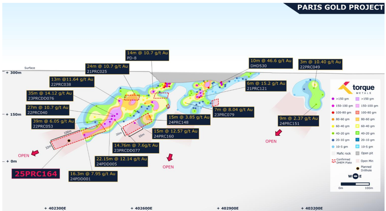
Figure 2 Paris deposit EM conductor plates modelled from DHEM surveys vectoring extensions of gold-associated sulphide minerals. Note recently surveyed holes show strong correlation between DHEM conductors and previously identified high grade gold mine
