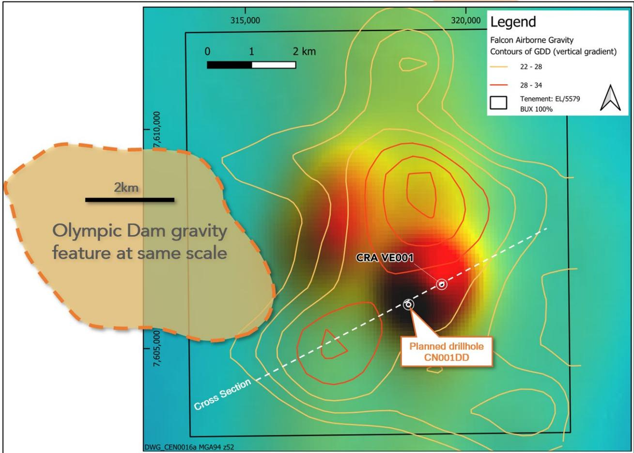
**Figure 3:** Centurion Project showing GSWA’s statewide magnetic imagery overlain with GSWA gravity contours along with the site of CRA’s VE001 which was abandoned before reaching basement. The semi-coincidence of magnetic and gravity anomalies is characteristic of IOCG systems like Carrapateena and Olympic Dam.
