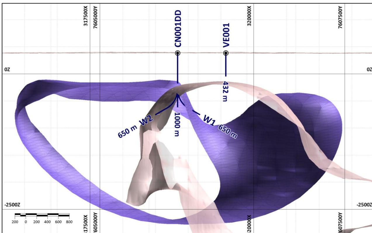
**Figure 2:** Cross section looking northwest with historic CRA drillhole VE001 and planned drillhole CN001DD. Wireframes are the gravity (purple) and magnetic (pink) inversions. "Daughter" holes W1 & W2 illustrate how the planned drill site allows for immediate follow-up drill testing of both the gravity and magnetic features utilising the initial 1,000 metre "parent" vertical hole.
